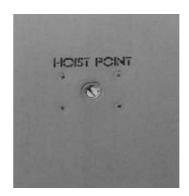
The words "HOIST POINT" were still visible and in the correct location. The fonts used for the words on the part matched those on the fan cowl of the aircraft.
