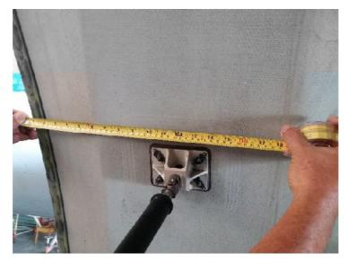
The dimension from the forward edge of the part to the start of the core ramp, which was 18 inches, was also consistent with that of the fan cowl on the aircraft, as shown in the above figure.
